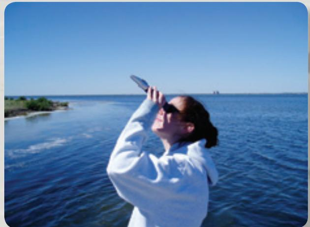
*Measuring salinity using a refractometer.*
